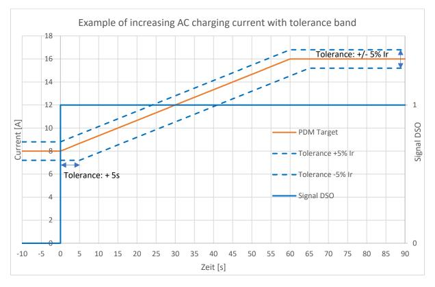
Diagram 3: Tolerance bands for AC charging current changes (example)
