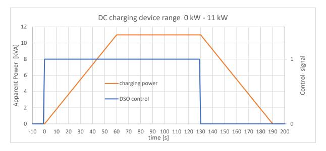
Diagram 4: Behaviour DC CD in the range between 0 kW and 11kW
