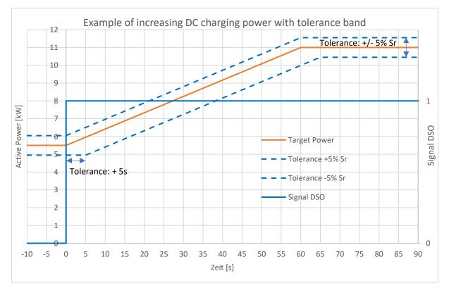
Diagram 5: Tolerance bands for DC charging power changes (example)
