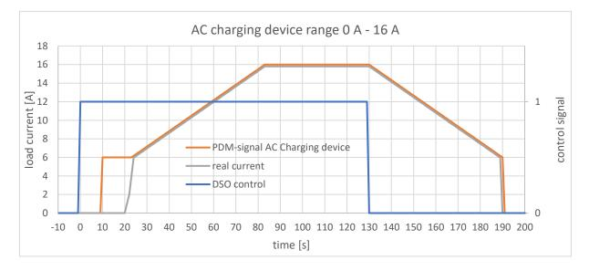
Reaction time: Ramp starts immediately – max. time delay 5 s.
